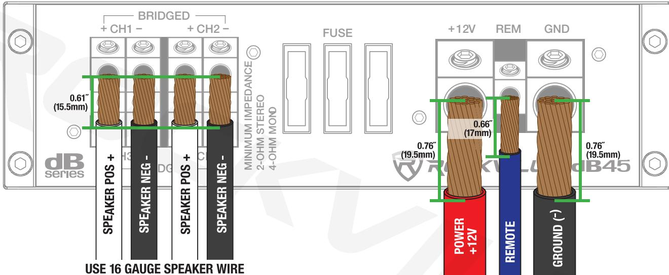
**TERMINAL DIAMETER:** POWER =  $\Phi$  0.33in (8.5mm), REM =  $\Phi$  0.15in (4mm), SPEAKER =  $\Phi$  0.15in (4mm)
