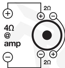
**TWO 2Ω DVC WOOFERS = 2Ω LOAD**
