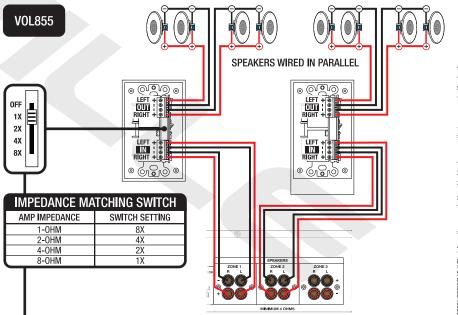
The VOL855 features an impedance matching switch which will allow to match your amp's minimum impedance, regardless of the number of speakers you use and their final impedance. For example, if your amplifier has a minimum impedance of 4 ohms and your speaker's final impedance is 2 ohms, the impedance switch should be set to 2X,
