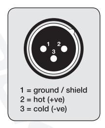
This microphone can be used for balanced and unbalanced applications. For balanced XLR connections use an XLR cable (included). For unbalanced connections use a 1/4" TS jack plug to a female XLR cable (not included). Be aware that when using a run longer than 16ft you may encounter humming caused by stray magnetic fields from power cables, lighting cables, and other electric appliances.
