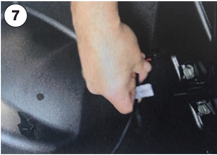
7. Route the speaker cable attached to the pod through the inside footwell 1/2" hole.
