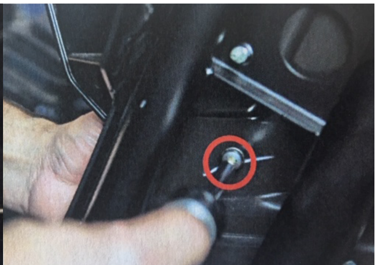
9. With the provided M6 screws and washers, loosely mount the pod through the 3 holes previously drilled. Once all screws have been inserted into the pod, hand tighten all 3 screws.
