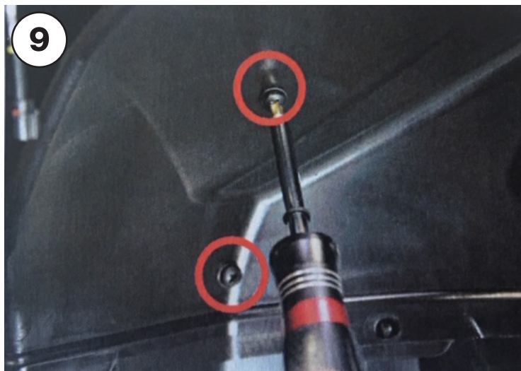
9. With the provided M6 screws and washers, loosely mount the pod through the 3 holes previously drilled. Once all screws have been inserted into the pod, hand tighten all 3 screws.
