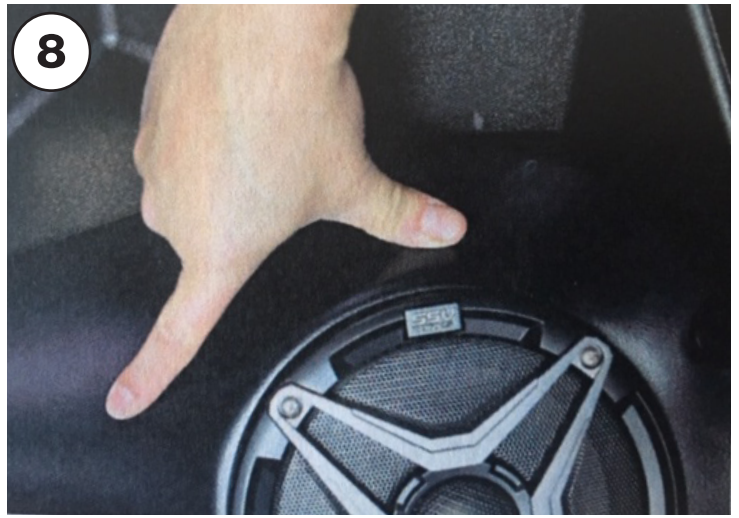
8. Position the speaker pod in place and line up with the drilled mounting holes.
