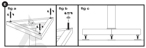
To place the stand on a carpeted floor, use the metal isolation spikes. Attach the spikes to the bottom of the base plate (fig a). If needed, adjust the spike height to keep the stand level. Use the washer and nut to secure the spike in the desired position (fig b). Place a metal disk underneath each spike to protect the surface on which the stand is placed (fig c).
