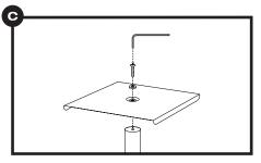
Hold the telescoping shaft vertically with the locking mechanism on top. With the indentation facing down, align the platform so that the indentation sits in the opening of the shaft. Insert a short screw and washer through the opening. Use the Allen key to tighten the screw. Do not overtighten.
