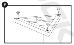
If you are placing the stand on a wood, laminate, tile, or bare floor you should use the included rubber feet. To install, simply push them into the holes at the bottom of the base plate.
