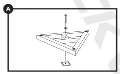
Turn the triangular base so that the insertion points for the rubber feet/steel spikes are facing up. Insert a long screw and washer through the opening on the base and through the opening in the shaft mounting plate. Push the plate against the base so that it fits snugly.
