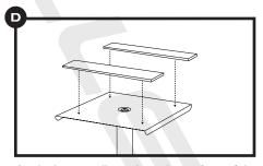
Apply the non-slip pads to the surface of the platform by removing the covering on the adhesive and carefully placing it onto the surface. Firmly smooth it out.
