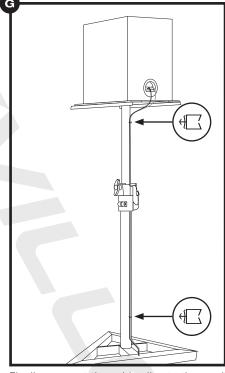
Finally, connect the cable clips to the small holes found on the rear of the stand. There is one just underneath the speaker platform and one near the base. Once they are in place, guide the speaker wires through the top clip, then along the telescoping shaft to the bottom clip. This will help keep the speaker cables tidy and out of the way.
