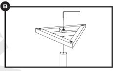
Turn the telescoping shaft 180 degrees and rest it on the platform. Align the end of the bolt (that was placed through the base plate and mounting plate) with the screw whole on the shaft. Use the Allen key to tighten the screw. Do not overtighten.
