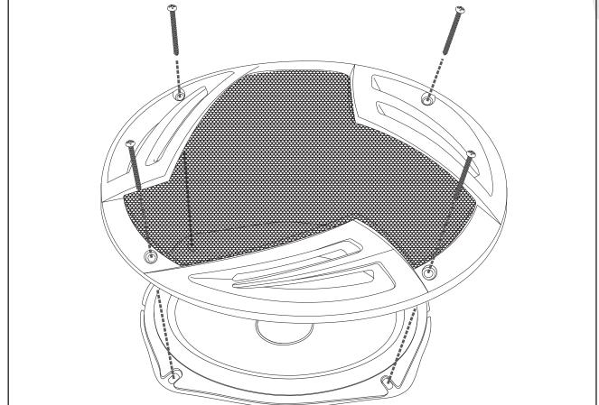
To install the speaker, slide the long screws through the holes in the grill and through the corresponding holes in the speaker.
