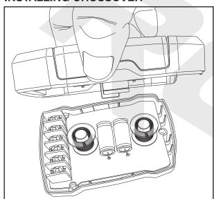
Remove the crossver's cover by pressing on either side of the cover and pulling up gently.
