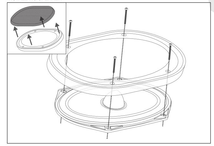
To install the speaker, remove the grille from the grille frame (see inset). Now, slide the long screws through the holes in the grill frame and through the corresponding holes in the speaker.
