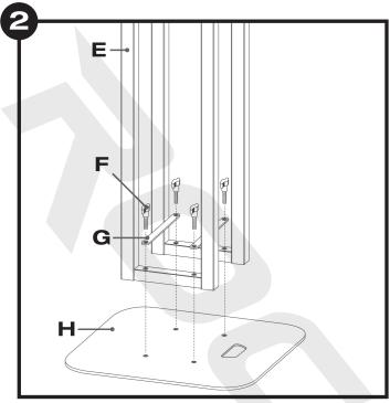
Attach the base plate (H) to the base support legs (E) using 4 of the hand tightening screws (F). Optionally you may use the included standard bolts. Make sure the cross brace supports (G) are inserted between the hand tightening screws and the base support legs as shown in the diagram above.
