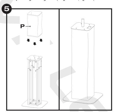
Finally, carefully guide the black or white (pictured, fig P) scrim over the unit. The scrim will fit the unit when fully extended and was designed to be folded or rolled over when using the stand at lower heights.
