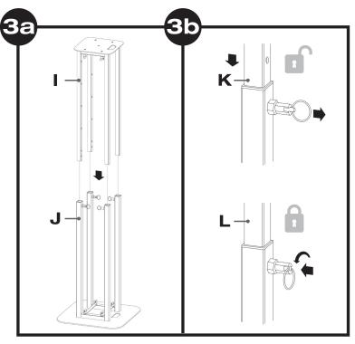
Ensure that all four height adjustment mechanisms are unlocked by pulling the pins out and rotating the rings (diagram 3b, figure L) Now slide the top plate assembly (I) onto the base plate assembly (J) as shown in diagram 3a. Lock the unit at the appropriate height by engaging the adjustment pins in the appropriate holes of the top support legs and close the locks by turning the rings 90° (diagram 3B, figure L).
