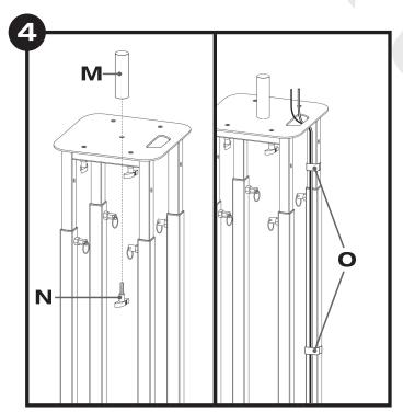
At this point you may apply the EVA foam pads (if needed) or attach the 35mm speaker adapter (M) using the remaining hand tightening bolt (N). Additionally you can use the included hook and loop fastener cable ties to guide any cables along the stand legs and through the handle cutout in the top plate (0).
