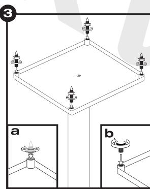
To place the stand on a carpeted floor, use the brass isolation spikes. Screw the spikes to the corresponding openings at each corner of the bottom of the base plate. Adjust the height as needed to keep the stand level. Use the nut to secure the spike's position (inset a). For wood, laminate, tile, or bare floor, use the included rubber feet (inset b).
