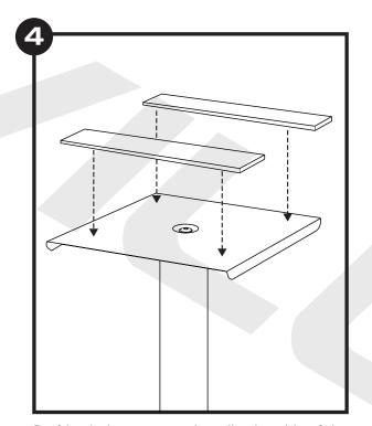
Peel back the cover on the adhesive side of the EVA sound isolation pads. Carefully place one on each side of the top plate and firmly smooth them out.
