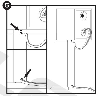
The final step is to feed the speaker cable into the u-shaped opening on the top of the stand body where it meets the top plate (see top inset) and bring it back out through the u-shaped opening at the bottom where it meets the base plate (see bottom inset).
