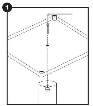
First, remove the socket head screws from the ends of the stand body. Turn the base plate upside down and align the hole in the center of the base plate with one of the holes on either end of the stand body. Insert a screw and use the Allen key to tighten it. Do not overtighten.
