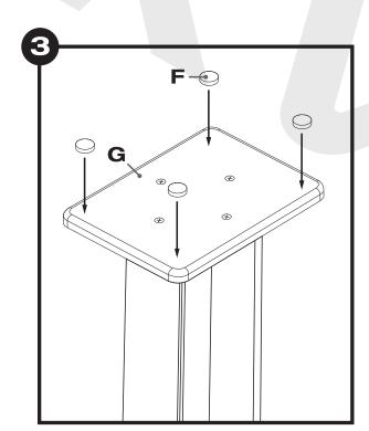
Peel back the cover on the adhesive side of the EVA sound isolation pads (F) and place one on each corner of the top plate (G). These pads help to minimize resonance.
