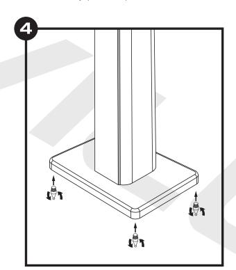
Now attach the isolation spikes to the bottom of the base plate. If needed, adjust the spike height to keep the stand level. To place the stand on a carpeted floor, use the brass spikes. If you are placing the stand on a wood, laminate, tile, or bare floor you should use the included rubber spikes.
