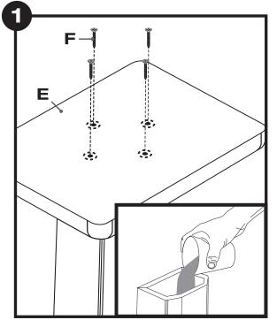
Attach the base plate (E; flat side up) by aligning the screw holes with the stand body as in figure 1. Use four screws (F) to secure it in place. After attaching the base plate you may consider partially filling the stand body with sand for additional stability (see inset).
