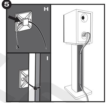
The final step is to attach the cable clips to the back of the unit. Peel the cover off of the adhesive backing and place the clips in the desired locations. Once the clips are in place, slide a zip tie through the opening on the side of the clip (see inset H). Use the zip tie to secure the speaker cables (see inset I).
