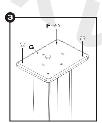
Peel back the cover on the adhesive side of the EVA sound isolation pads (F) and place one on each corner of the top plate (G). These pads help to minimize resonance.
