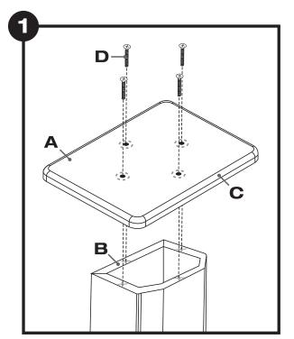
Select the appropriate size platform (A; there are two included). Align the holes on the platform with the edges of the stand body (B). Make sure that the beveled side of the platform (C) is facing up. Use four screws (D) to secure it in place.
