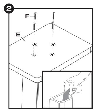
To attach the base plate (E; flat side up), align the screw holes with the stand body as in figure 1. Use four screws (F) to secure it in place. Before attaching the plate you may consider partially filling the stand body with sand for additional stability (see inset).
