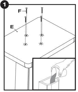
Attach the base plate (E; flat side up) by aligning the screw holes with the stand body as in figure 1. Use four screws (F) to secure it in place. After attaching the plate you may consider partially filling the stand body with sand for additional stability (see inset).
