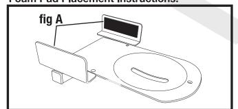
Apply one of the 4 included foam pads to the inside of the side supports of each speaker platform as shown in figure A.
