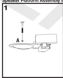
Slide a locking bolt through the opening at the top of the speaker platform (A).
