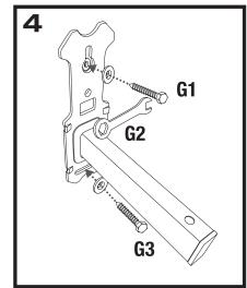
Place the wall bracket into position over the holes and insert the top carriage bolt with the small washer (G1). Tighten the carriage bolt with a wrench (G2) or use a drill with a 13/32" socket bit. Insert the second screw (G3). Use a level to ensure that the bracket is properly aligned. Now tighten the carriage bolt. Keep the level next to the bracket to ensure that it stays aligned.
