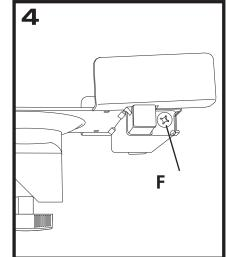
Once the bolt is all the way through, slide on a To extend the side supports, use the screws large washer (C). Screw the locking knob onto the located underneath the them (F). There is one on protruding part of the locking bolt (D). Do not either side. Use a Phillips head screw driver to turn tighten completely. Adjust the angle and direction the screw counter-clockwise to extend and
