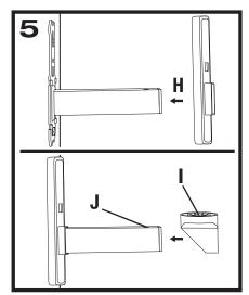
Slide the bracket cover onto the bracket arm and push back onto the base until it clicks into place (H). Now slide speaker platform support onto the end of the mounting bracket arm as shown. Align the hole in the speaker platform support (I) with the hole in the mounting bracket arm (J).
