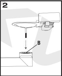
Align the bolt with the hole in the speaker platform support (B) and slide it through. The convex bottom of the speaker platform should rest snugly on the support piece.
