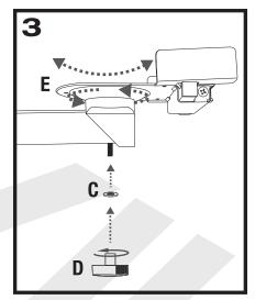
of the speaker platform by tilting it or turning it to clockwise to retract. the desired position (E). Once it is properly adjusted, you may fully tighten the locking knob.
