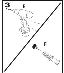
Using a drill and a 11/32" bit, make a hole where you made your first mark (E). Repeat for your second mark. We recommend realigning the holes with the bracket and releveling it, to make sure everything is aligned. If you are using the anchors, make sure the holes are deep enough to accomodate them. Insert the anchors (F) and tap in with a hammer if needed.
