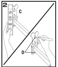
Press the plate of the bracket up against the wall so that it's flush. Make sure it's level using a torpedo or small level (C). Place a mark at the top and bottom openings where your anchor holes will be (D). If you are drilling into a stud, the anchors are not necessary.
