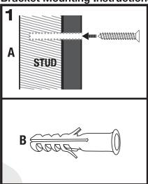
Determine an area to mount the bracket. We recommend mounting it to a wood stud (A). If you must mount it on drywall, use the included wall anchors (B). Be sure that they are properly installed.
