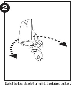
Tighten the hex bolt to lock it in place.
