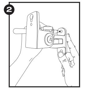
Place a mark at the top and bottom openings where your anchor holes will be. If you are drilling into a stud, the anchors are not necessary.
