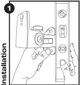
Press the bracket up against the wall so that it's flush. Make sure it's level using a torpedo or small level.
