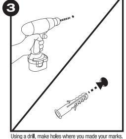
Ensure your holes properly align with the bracket. If you are using the anchors, ensure the holes are deep enough to accomodate them. Insert the anchors and tap in with a hammer if needed.
