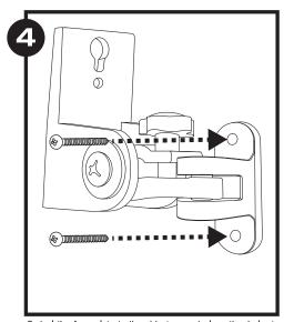
Swivel the face plate to the side (see swivel section below). Place the wall bracket into position over the anchors and insert a wall screw into the top hole. Do not fully tighten. Use a level to ensure that the bracket is properly aligned. Fully tighten the screw. Now, insert and tighten the second screw.
