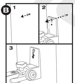
If your speakers have a mounting screw, partially unscrew it (1) and slide it through the bracket's mounting hole (2). Gently push down to ensure it has settled into the narrow part of the mounting hole (3). If the speakers have no mounting screws, use the M6 long screws.
