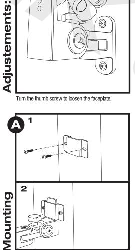
If the speaker has no mounting holes or screws, use the included u-shape bracket and bracket screws. Attach the bracket to the back of the speaker (1) and then slide it onto the face of the bracket (2).
