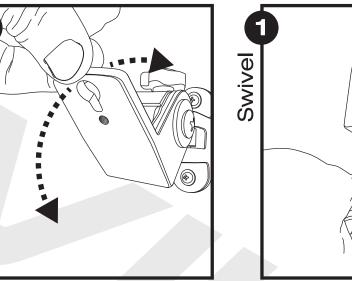
Tilt the faceplate up or down to the desired angle. Turn the thumb screw to lock the position.
