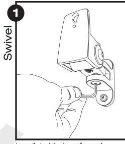
Loosen the hex bolt using an allen wrench.
