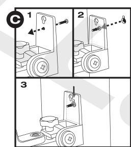
For speakers with a mounting hole, partially screw the M5 short screw into the small hole on the face of the mounting bracket (1). Mount the speaker onto the screw (2). Gently push down to ensure it has settled into the narrow part of the speaker's mounting hole (3).
