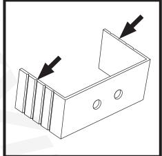
5. Fasten the bracket to the remote control unit using the washers and bolts as shown in the illustration. Do not overtighten the bolts.
