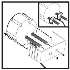
4. If the bracket arms are too long, adjust the length by using an appropriate tool to remove the necessary amount of breakaway segments.
