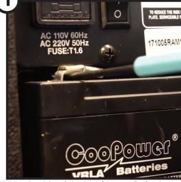
Using the pick tool (you can also use a flat head screwdriver or a butter knife), gently hook into the negative terminal of the battery.
