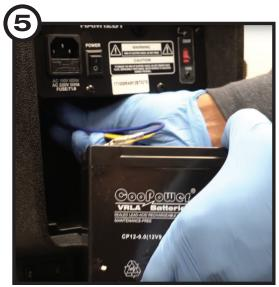
Carefully tuck the wires into the battery compartment before re-inserting the battery.
