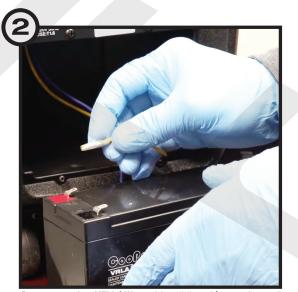
Reconnect the YELLOW positive (+) cable to the red positive (+) terminal of the new battery.
