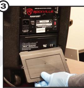
Once the bottom of the cover is out, gently pull down and away. Set the cover aside.
