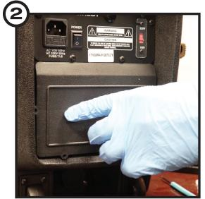
Once the tabs are in place, gently press the bottom of the back plate ensuring that it is properly seated.
