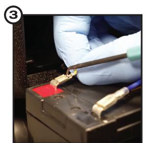
Use the pick tool to release the YELLOW positive (+) cable from the terminal. Simply push down on the small tab (shown above) and pull the cable.
