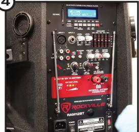
Before re-inserting the battery, perform a quick power-on test to ensure everything is correctly connected. If everything is in proper working order, proceed to the next step. Otherwise, please repeat the steps in the "Replacing the Battery" section of this instruction sheet. MAKE SURE TO UNPLUG THE UNIT BEFORE PROCEEDING.
