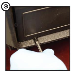
Take the four screws and tightly fasten them in so the back plate is secure. Do not over tighten.
