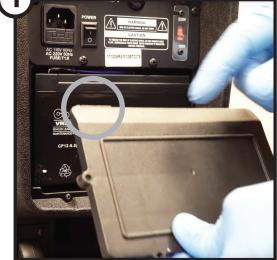
Replace the back plate by inserting the top of the plate first, ensuring that the plastic tabs (cirlcled in the image above) slide into the correpsonding slots located below the bottom of the amp plate.
