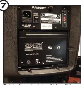
The battery is properly seated once it is flush with the outer edge of the battery compartment as shown in the image
