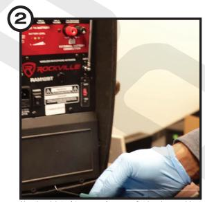
Use the pick tool (you can also use a flat head screwdriver or a butter knife) to carefully pull the bottom of the battery cover.
