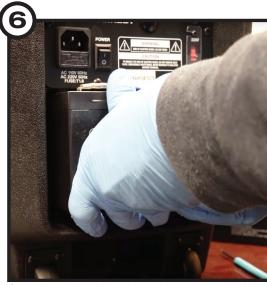
Gently insert the battery into the compartment being careful not to pinch the cables.
