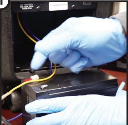
Remove the plastic terminal covers on the new battery.
