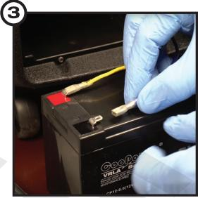
Reconnect the BLUE negative (-) cable to the black negative (-) terminal of the new battery.
