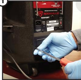
Remove the 4 screws that hold the battery cover in place using a Phillips head screwdriver. MAKE SURE THE UNIT IS UNPLUGGED BEFORE REMOVING THE SCREWS.
