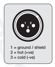
This microphone can be used for balanced and unbalanced applications. For balanced XLR connections use the included XLR cable. For unbalanced connections use the included 1/4" TS jack plug to female XLR cable. Be aware that when using a run longer than 16ft you may encounter humming caused by stray magnetic fields from power cables, lighting cables, and other electric appliances.
