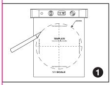
Using the included template, cut an opening in the drywall.
