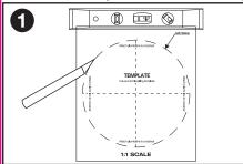
Using the included template, cut an opening in the drywall.
