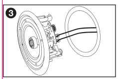
Connect the speaker wires. Be sure to observe proper polarity.
