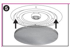
Replace the grill by gently pushing it onto the speaker face.
