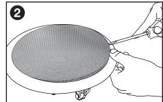
To remove the grille insert a flat head screwdriver into the space between the grill and the inner lip of the speaker housing. Gently lift the grill out being careful not to bend it.
