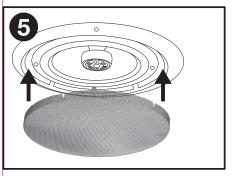
Replace the grill by gently pushing it onto the speaker face.
