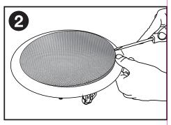
To remove the grille insert a flat head screwdriver into the space between the grill and the inner lip of the speaker housing. Gently lift the grill out being careful not to bend it.
