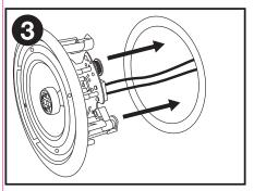
Connect the speaker wires (be sure to observe proper polarity), set taps to the desired power setting (see diagram on the facing page), and insert the speaker into the cutout.
