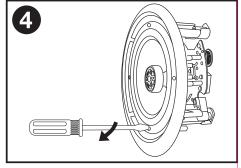
Screw down each of the four Phillips head screws. The locking tabs will swivel into place and secure the unit to the rear surface of the drywall. Put in the strips of adhesive to secure the crille.
