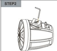
After loosening the two screws and determining the optimal angle for your speakers on the mounting bar, tighten the two screws in place to secure the metal base of the mounting ring tightly.
