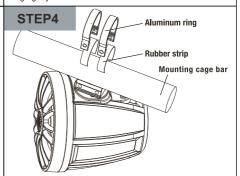
Determine the mounting cage bar size and place the appropriate rubber strip around it. This will ensure a proper it and prevent scratching. Push the aluminum ring over the bar. Align the aluminum rings with the metal base of the mounting rings on the waketower speaker.
