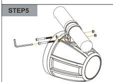
Secure the aluminum rings to the metal base using a pair of M6  $\times$  60mm screws, M6 flat washers, and M6 locknuts as illustrated. The locknut should be installed into the hexspaped recess on one end of each ring. Do not overtighten. To change the position of the speaker loosen the screws, adjust the speaker, then retighten the screws.
