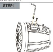
The two screws can be unbolted to loosen the metal base of the mounting ring to adjust the mounting angle. Make sure to put all components of the mounting hardware in a safe location.
