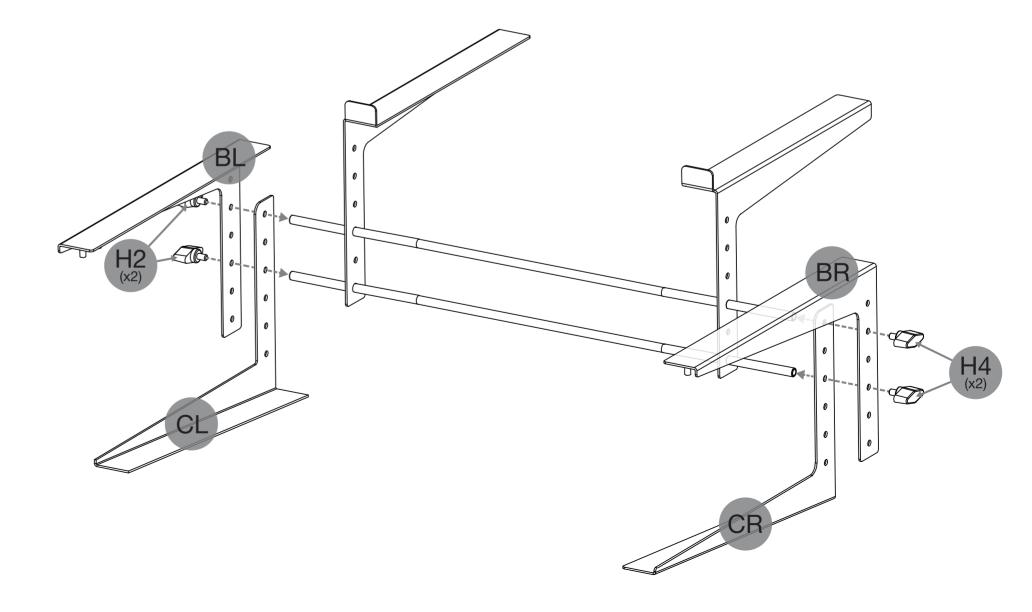
4. Assemble bottom support rod using the remaining E1, E4, F1, G1, and G2 pieces: Additional washers are included and can be added as needed.
