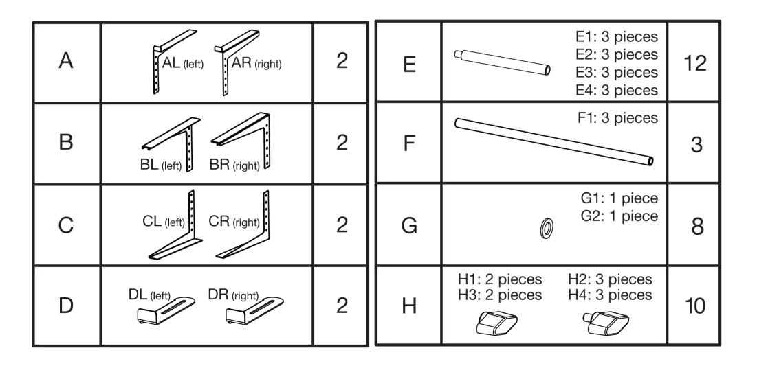
**1. Assemble central support rods:** screw one E3 piece to the left end and one E2 piece to the right end of the an F1 rod. Repeat this procedure with a second F1 rod. These will serve as the horizontal central supports. Once assembled, set them aside.
