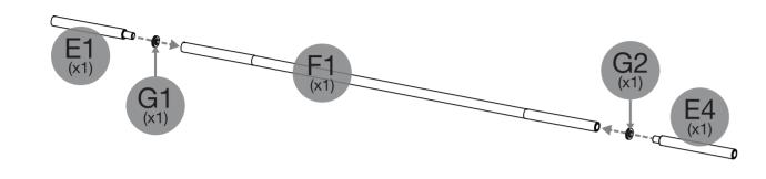
5. Connect bottom support rod to the bottom holes of the stand feet:
