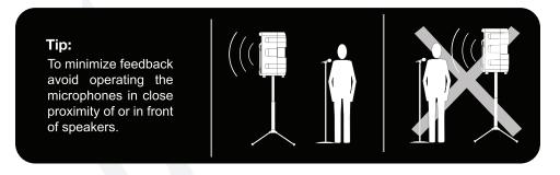
Feedback can also be caused by the acoustics of the venue. In these instances the proximity effect may cause feedback. In most cases, simply moving a little away from the microphone may resolve the issue.
