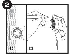
Align the left side of the bracket with a stud (C). Place a mark at the top and bottom left side openings as well as the top right opening (D).
