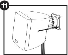
Insert the last screw into the lower right hand hole and tighten it.
