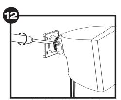
After making final orientation adjustments to the speaker, use a Phillips head screw driver to tighten the screw on the side of the molded nut to ensure the bracket is fixed in the desired position. Do not overtighten.
