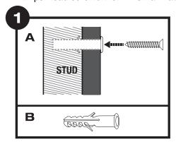
Determine an area to install the mounting bracket. We recommend mounting it to a wood stud (A). If you must install it on drywall, use wall anchors (B). Be sure that you have chosen the appropriate type and that they are installed properly.
