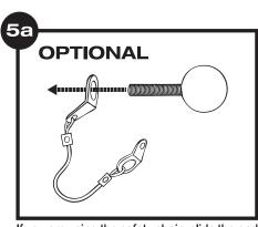
If you are using the safety chain, slide the end with the largest opening onto the ball shaft.
