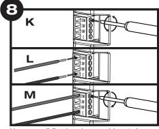
Use a small flat-head screwdriver to loosen the appropriate terminal screws (K). Strip a half inch of sheathing from the ends of the speaker wire. Insert them into the terminal openings (L). Be sure to observe proper polarity. Tighten the screws (M).
