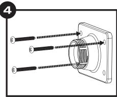
Use 3 of the included screws to secure the top left, bottom left, and top right corners of the bracket. If you are using anchors, ensure that you are using the proper screws for your anchor type.
