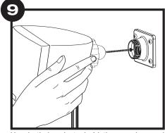
Use both hands to hold the speaker and gently push the ball into the wall bracket. Check that the ball is properly seated.
