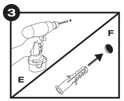
Drill holes where you made your marks (E). Ensure they properly align with the bracket. If using anchors, ensure the holes are deep and wide enough to accommodate them (F).
