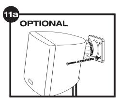
Insert the last screw into the open end of the safety cable. With the safety chain attached, insert the screw into the lower right hand hole and tighten it.
