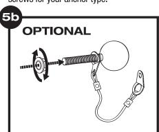
Thread the lock nut onto the shaft with the nut's round surface facing away from the ball. Tighten it all the way onto the threaded shaft, but do not tighten it flush with the ball.
