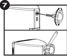
Screw the ball shaft/molded nut assembly into the threaded insert a the back of the speaker until it is fully seated against the opening (I). Use a wrench to tighten the nut and ensure it is completely flush with the speaker housing (J).
