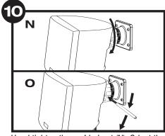
Hand tighten the molded nut (N). Orient the speaker in the desired direction. Insert the metal bar into one of the holes on the molded nut and tighten it to lock in the position (O). Do not overtighten.
