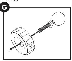
Slide the ball shaft assembly through the back of the molded nut.
