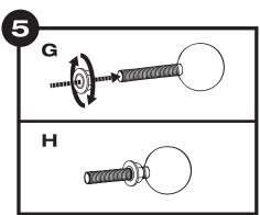
Thread the lock nut onto the shaft with the nut's round surface facing away from the ball (G). Tighten it all the way onto the threaded shaft as shown in the illustration above (H).
